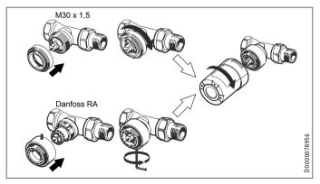
If required, use screws to attach an adaptor to the radiator valve.
