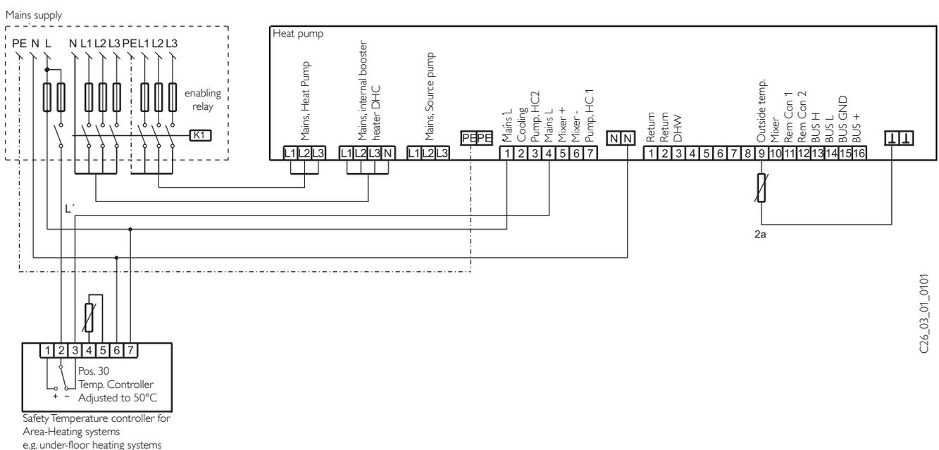
Safety Temperature controller for Area-Heating systems e.g. under-floor heating systems
