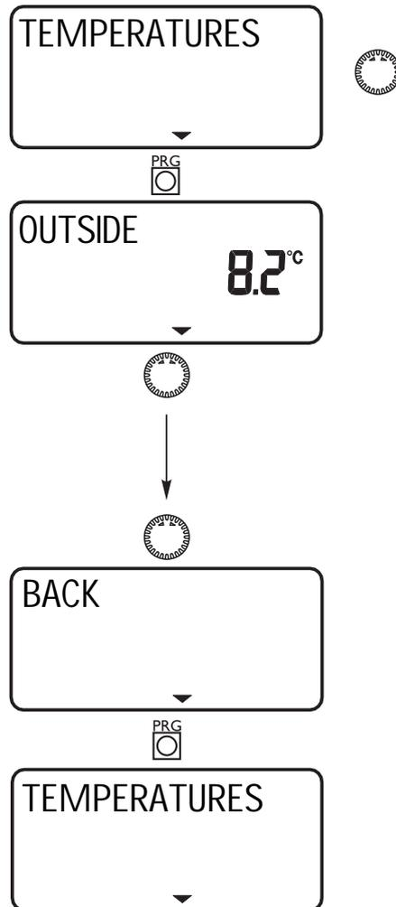
Note: Actual or set temperatures will not be displayed, if the corresponding sensor is not connected.
