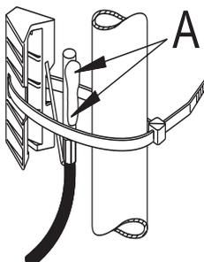
This sensor is required if a mixer circuit is installed. Installation information: Thoroughly clean the pipe. Apply heat transfer paste **A**, and secure the sensor with a cable tie.
